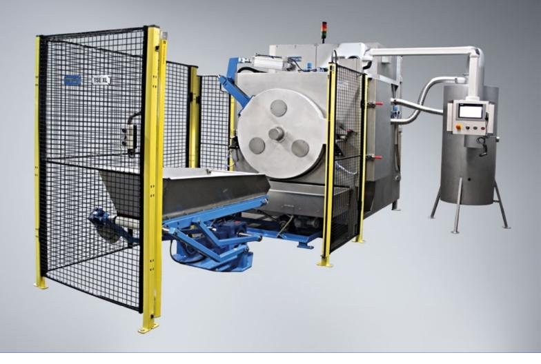
The drum-type media-blast deburring systems of the ROTOR TSE Premium series are designed for the cryogenic finishing of large batch sizes of tumbler-compatible rubber, plastic and non-ferrous metal molded parts.
