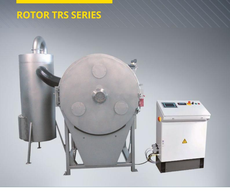
The ROTOR TRS series offers drum-type deburring systems for the cryogenic finishing of shape-, material-, and surface sensitive molded parts and seals made of plastics and rubber with a geometric drum volume of up to 700 litres.
